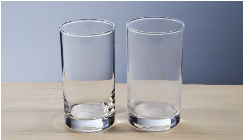
* Left: Glass tumbler without weathering Right: Glass tumbler with weathering
