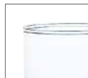
Burn-off (Hot-cut) with round ring
